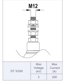
Bushing St. 1 Suitable for Low Voltage Side
