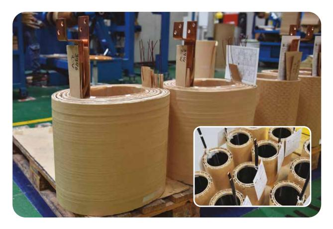
Both the primary and secondary windings are made of copper or aluminum. The primary voltage is directly wound on the secondary voltage winding, with insulating barriers and cooling channels between the two windings. Secondary voltage coils are rectangular wires or foil conductors. Primary voltage coils are round enamel wires, or rectangular paper insulated wires for high power ratings, or paper insulated round wires.
