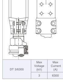
Bushing St.1 Suitable for Low Voltage Side
