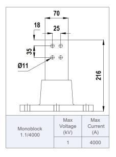
Bushing St. 1 Suitable for Low Voltage Side
