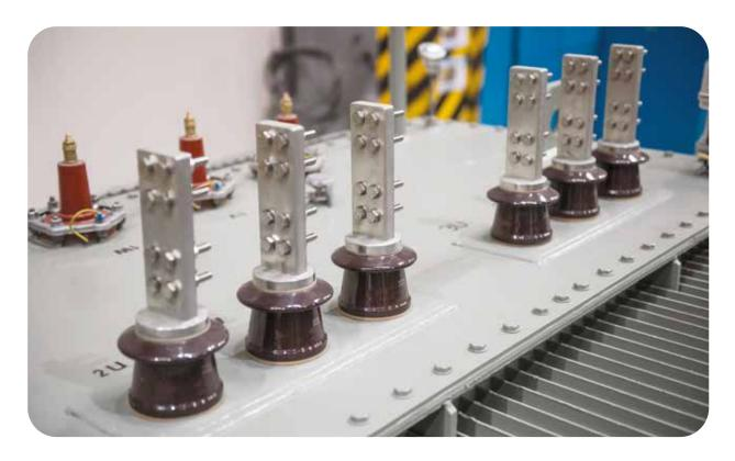
A dual voltage transformer can be defined as a transformer capable of providing two types of voltages, i.e. if the two separate windings are connected in series, they will provide the sum of voltages supplied to the two coils and if the two windings are connected in parallel, then the net voltage will be decreased. These voltages can be switched within the transformer according to the type of output required by using a dual voltage switch.
