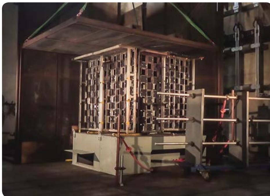
Figure 16: A Picture Taken During the Internal Arc Test of 17,5kV SFA-RM
