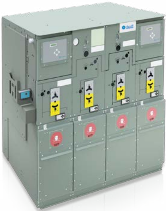
Figure 3: 17.5 kV, 2 ring switches / up to 630A + 2 vacuum circuit breakers / up to 630A; front view and single line diagram
