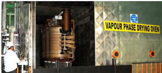
VPD is used in drying of cellulosic insulation of the transformer winding which requires that the moisture content be brought to 5 ppm levels before impregnation of the winding with transformer oil, recovery of the oil and discarding the moisture. The fluid basically acts as a heat carrier to the insulation.
