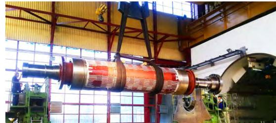
The life of a generator is mainly dependent on the life of its insulation. Therefore the aging process of the generator has to be very closely monitored. Just like the pulse rate, the blood pressure, sugar level etc., of a human are indicative of his health condition, the capacitance, leakage current, dissipation factor, polarization index, surge voltage with standing strength and partial discharge factors are indicative of the insulation condition of an electric rotating machine.
