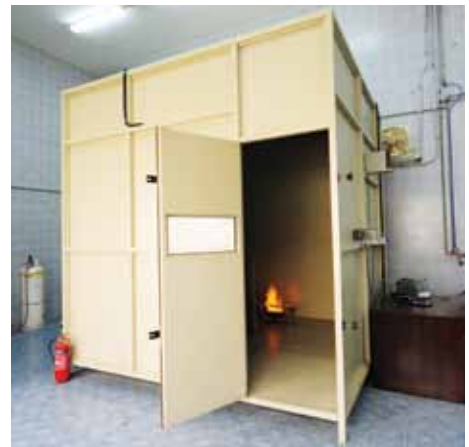
Smoke density 3 m test cube (IEC 61034)
