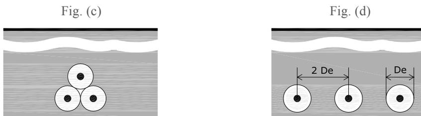
The cable depth is measured to the cable axis or to the centre of the trefoil group.
