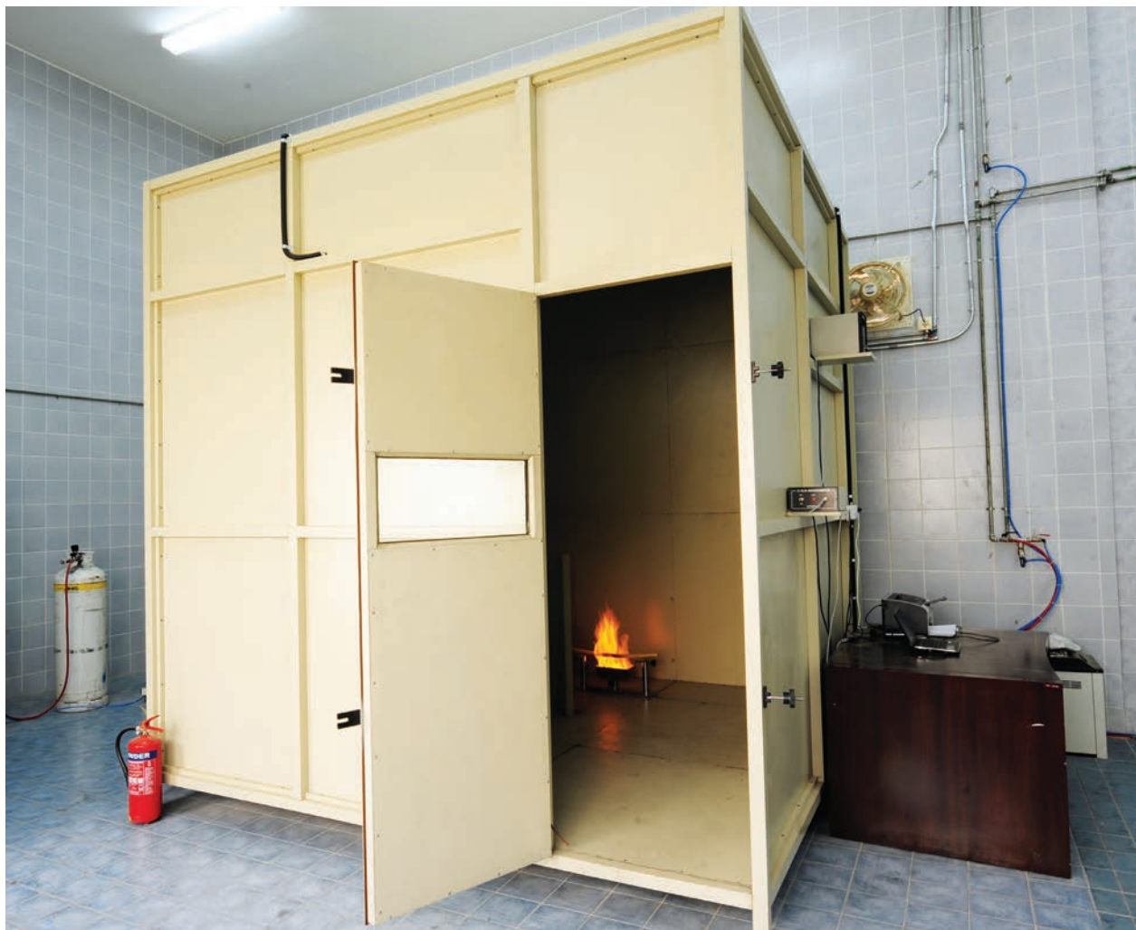
Smoke density 3 m test cube (IEC 61034)
