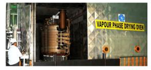
VPD is used in drying of cellulosic insulation of the transformer winding which requires that the moisture content be brought to 5 ppm levels before impregnation of the winding with transformer oil, recovery of the oil and discarding the moisture. The fluid basically acts as a heat carrier to the insulation.
