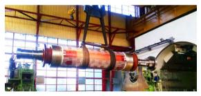
The life of a generator is mainly dependent on the life of its insulation. Therefore the aging process of the generator has to be very closely monitored. Just like the pulse rate, the blood pressure, sugar level etc., of a human are indicative of his health condition, the capacitance, leakage current, dissipation factor, polarization index, surge voltage with standing strength and partial discharge factors are indicative of the insulation condition of an electric rotating machine.
